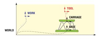
Absolute moves and positions are defined in the work coordinate system. Incremental moves can be done in the tool or in the work coordinate systems.
