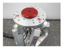
To avoid damages, the HXP50V6-MECA is delivered with a locking system that includes a center rod and a clamping wheel.
