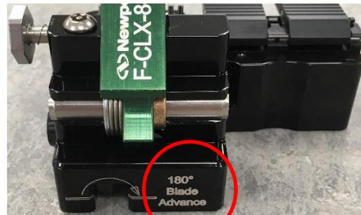
This is shown underneath by a scale printed on the blade advance block (see green circle). The blade is 3.5mm long and so there are up to 10 positions on each blade.
