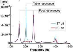
FIGURE 3. The influence of active damping of a table on transfer dynamic compliance from the table to the top of the post. Transfer dynamic compliance estimates the ratio of the horizontal acceleration on the top of the post (recalculated into displacement) to the vertical force on the table, as a function of frequency.
