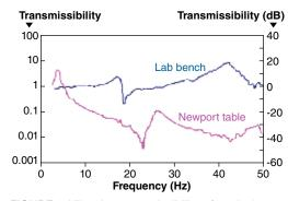
FIGURE 4. Vibration transmissibility of vertical floor motion is greatly improved with a Newport pneumatic isolation workstation compared to a typical built-in laboratory bench. (*Courtesy of Amick and Stead, Meeting of the ASA, 2002*)
