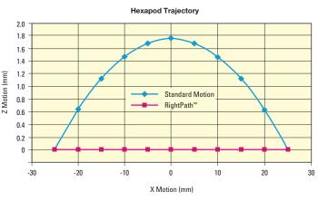
RightPath<sup>™</sup> Trajectory Control enables minimal runout in linear and arc trajectories.
