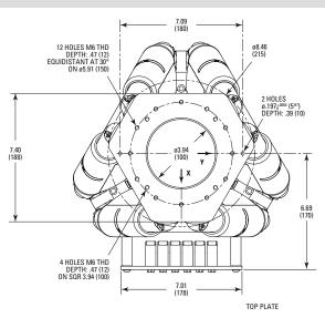
MODEL SHOW: HXP200-MECA DIMENSIONS IN INCHES (AND MILLIMETERS)
