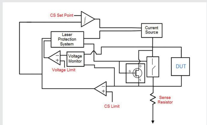
Figure 1- Schematic diagram of the LDP-3830 laser protection system circuitry
