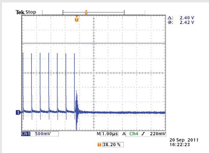
Figure 6: Screen capture of 1kV EFT event on the AC power line.
