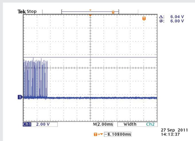
Figure 5: Loss of power or brown out turn off.
