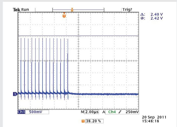
Figure 7: Screen capture during a 1kV surge event on the AC power line.
