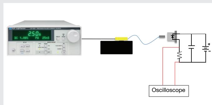
Figure 4: Schematic diagram of transient testing of the LDP-3830.
