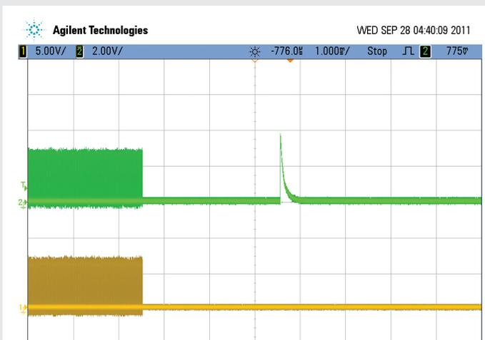
Figure 3: The fast shut down response of the LDP-3830. The yellow signal is the optical output and the green signal shows the current monitor
