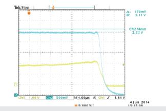
Figure 8: Intermittent contact response of the LDC-3736 with appropriate voltage limit setting
