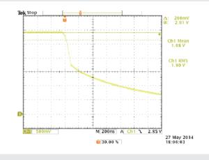
Figure 5: LDC-3736 laser current disabled due to loss of power or brown out
