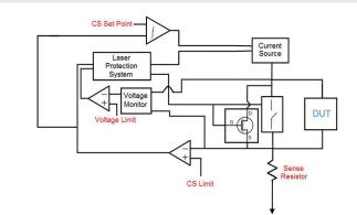
Figure 1- Schematic diagram of the LDC-3736 laser protection system circuitry
