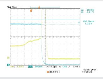
Figure 9: Intermittent contact response of the LDC-3736 with improper voltage limit setting
