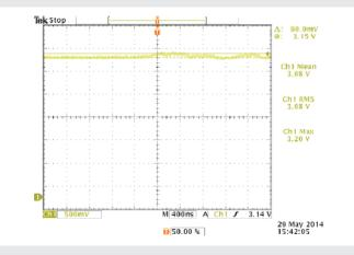
Figure 7: Effect on laser output due to 1 kV power surge event on AC power line
