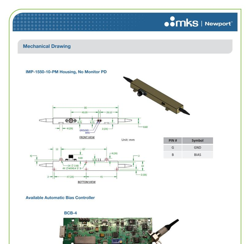
The BCB-4 is a compact bias control board designed for M-APE-I-1550-20 modulator
