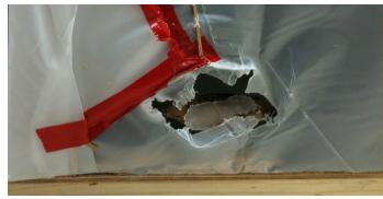
Shipping crate with a hole in the side caused by a forklift
