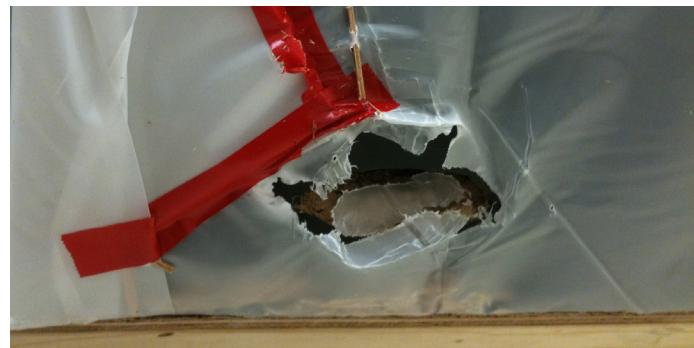
Shipping crate with a hole in the side caused by a forklift
