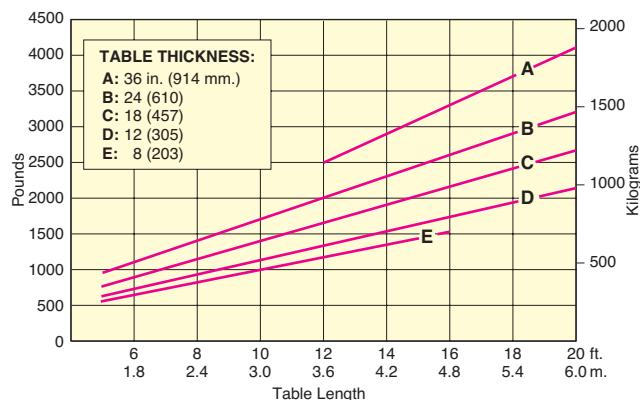
Figure 1: Approximate net weights ( $\pm 10\%$ ) for 4 ft (1.2 m) wide steel tables. For 5 ft (1.5 m) wide models add 20%, for 3 ft (0.9 m) models, subtract 25%. Shipping weights can be estimated by adding 100–200 lbs (45–90 kg) for crate weight.
