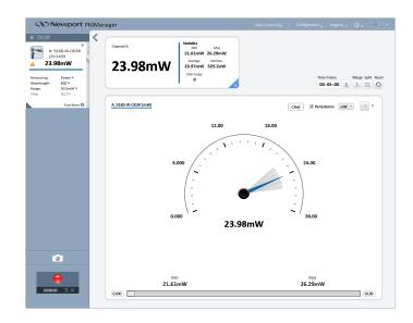
845-PE-RS with 918D Photodiode sensor and PMManager showing power needle screen
