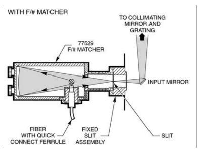
Figure 26: F Number Matcher Used with Fiber Optic Cable.
