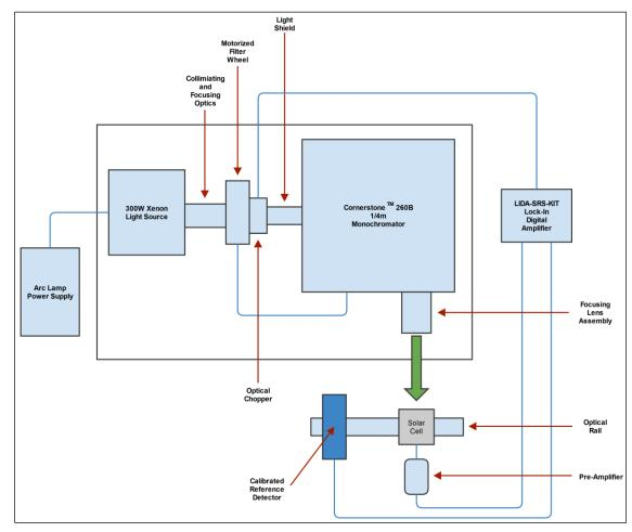
Figure 4: Application Example: Quantum Efficiency Measurements.
