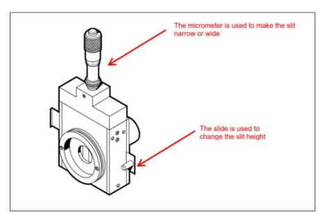
Figure 10: A Micrometer Adjustable Slit.
