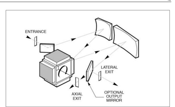
Figure 1: Optical Configurations of the Cornerstone 260B with Quad Grating Assembly.
