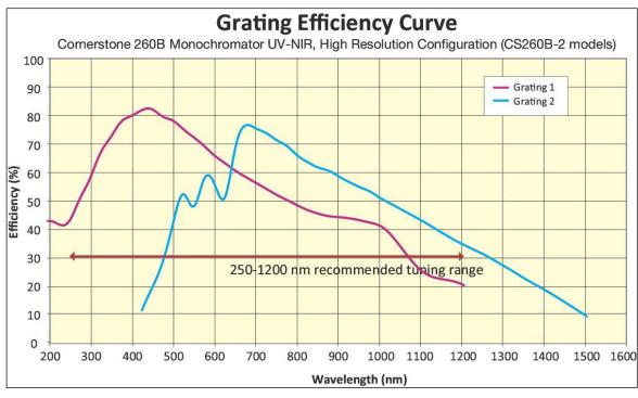
Figure 18: Grating Efficiency Curve, Cornerstone 260B Monochromator UV-NIR, High Resolution Dual Configuration (CS260B-2 Models).
