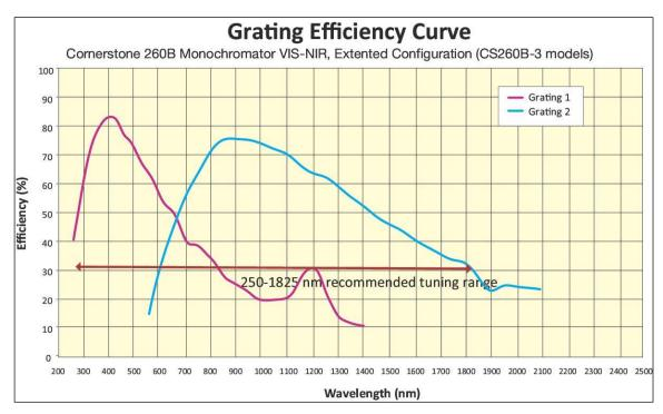
Figure 19: Grating Efficiency Curve, Cornerstone 260B Monochromator VIS-NIR, Extended Range Configuration (CS260B-3 Models).
