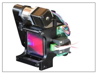
Figure 15: Gratings Installed on quad mount.
