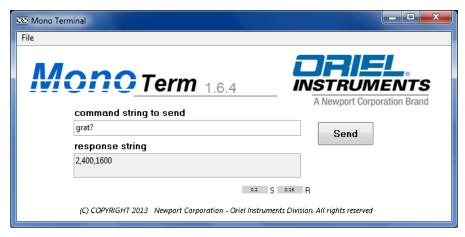
Figure 311: Query Using MonoTerm Software.
