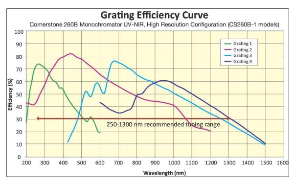
Figure 17: Grating Efficiency Curve, Cornerstone 260B Monochromator UV-NIR, High Resolution Quad Configuration (CS260B-1 Models).
