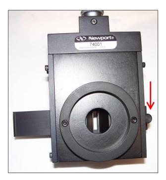
Figure 13: Tallest Micrometer Adjustable Slit Height.
