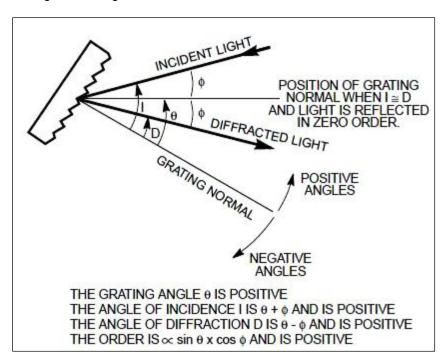
Figure 411: Sign Convention for the Angle of Incidence, Angle of Diffraction and Grating Angle
