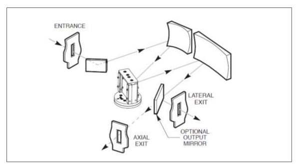
Figure 2: Optical configuration of the Cornerstone 260B with Dual Grating Assembly.
