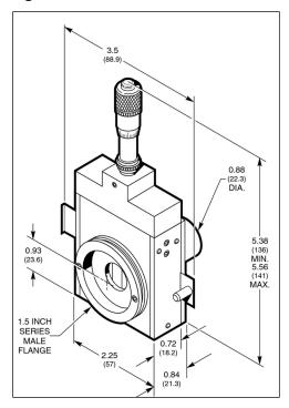
Figure 34: Micrometer Adjustable Slit Dimensions
