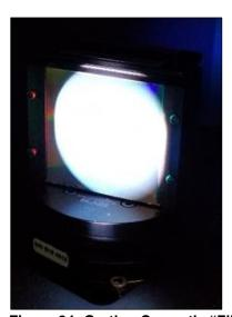
Figure 24: Grating Correctly "Filled" with Light.
