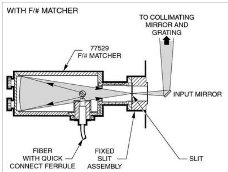
Figure 26: F Number Matcher Used with Fiber Optic Cable.
