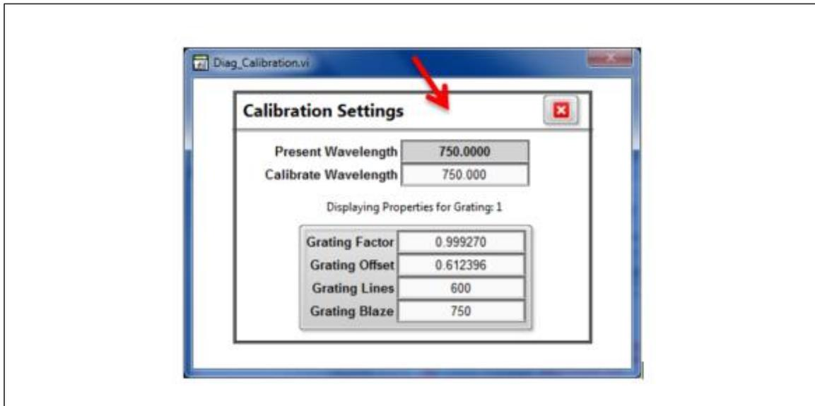
Figure 32: Entering Calibration Values in Utility Software.
