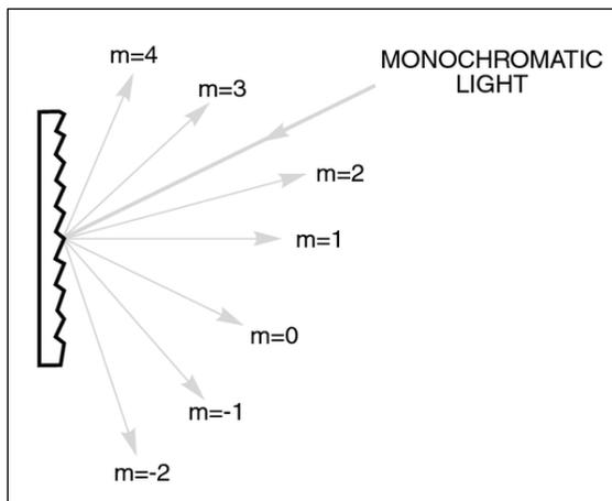
**Figure 399: The Grating Equation Satisfied for a Parallel Beam of Monochromatic Light.**
