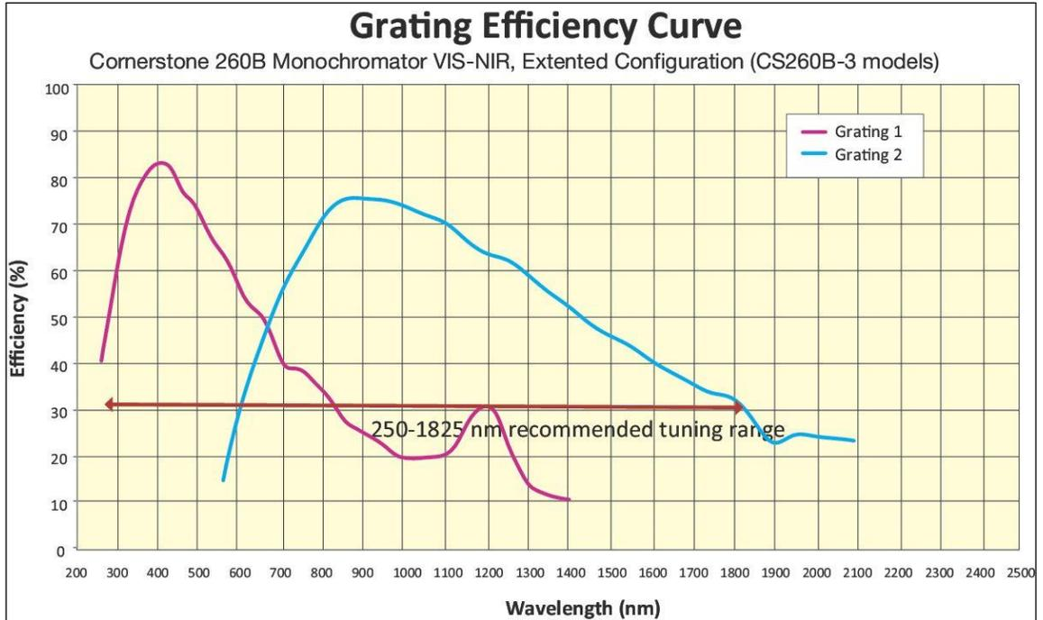
Figure 19: Grating Efficiency Curve, Cornerstone 260B Monochromator VIS-NIR, Extended Range Configuration (CS260B-3 Models).
