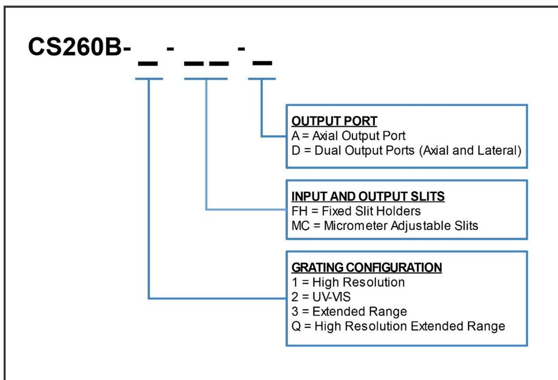
Figure 3: Model numbering system.
