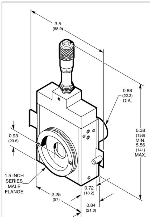
Figure 34: Micrometer Adjustable Slit Dimensions
