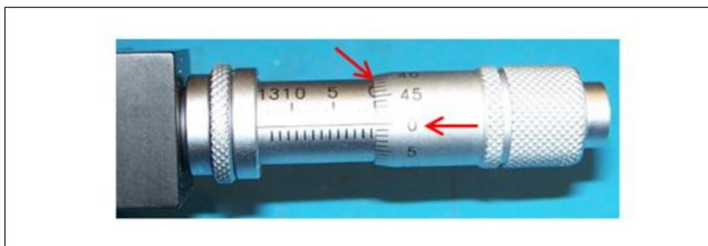
**Figure 11: A Fully Closed Micrometer Adjustable Slit.**
