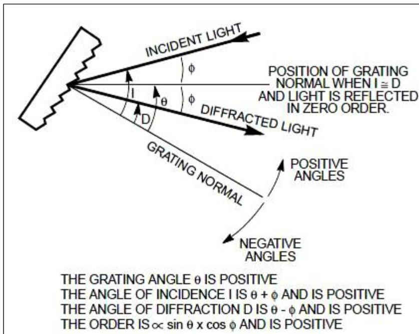
**Figure 411: Sign Convention for the Angle of Incidence, Angle of Diffraction and Grating Angle**
