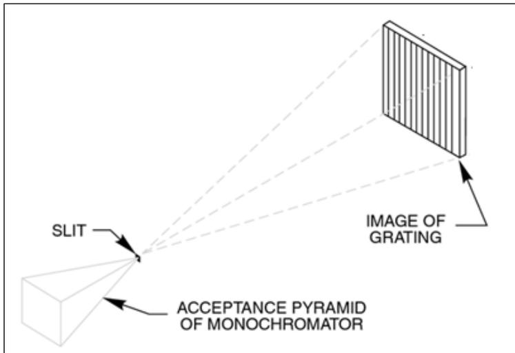
Figure 23: Acceptance Pyramid of Monochromator.
