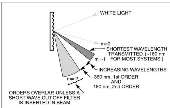
**Figure 40: Polychromatic Light Diffracted from a Grating.**
