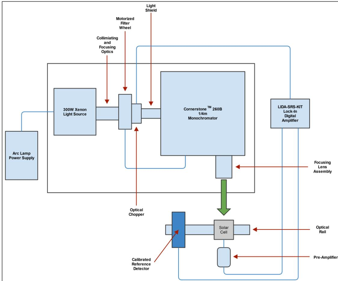
Figure 4: Application Example: Quantum Efficiency Measurements.
