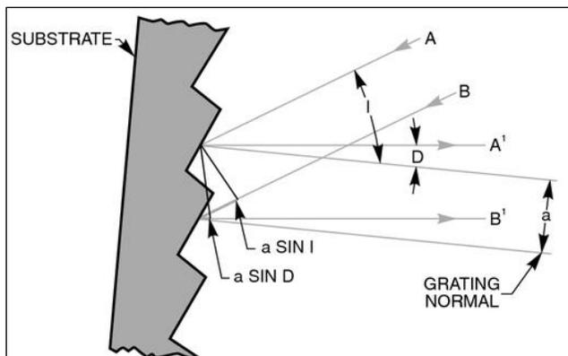
Figure 38: The Sawtooth Pattern of a Grating Section
