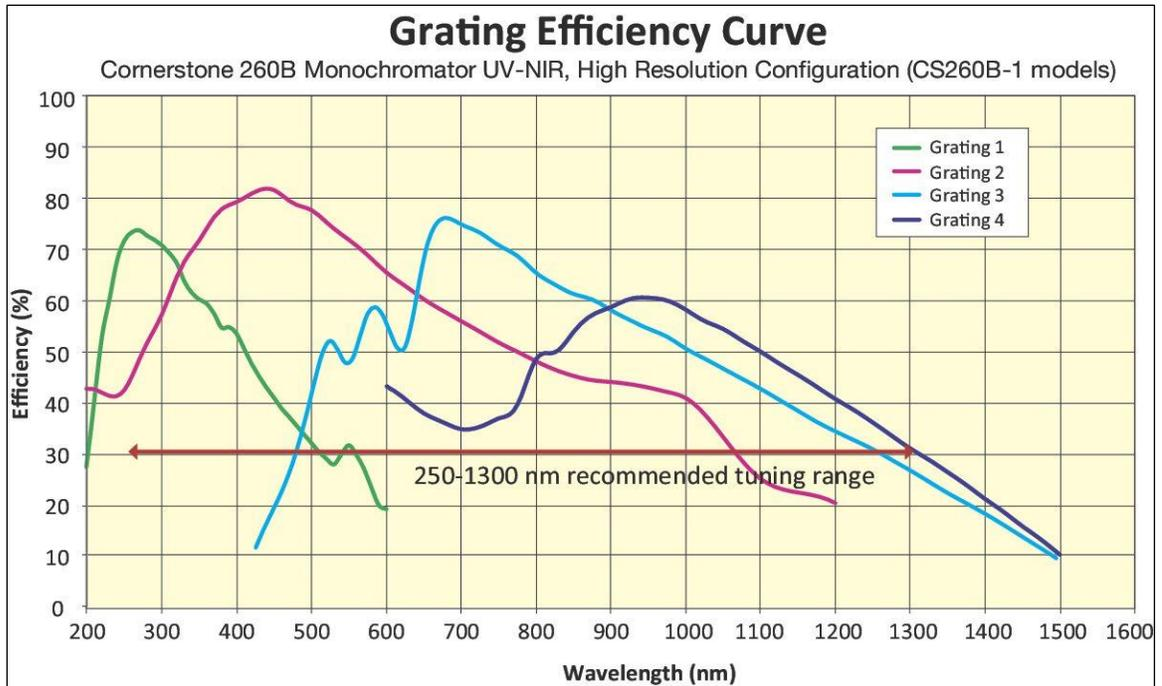
Figure 17: Grating Efficiency Curve, Cornerstone 260B Monochromator UV-NIR, High Resolution Quad Configuration (CS260B-1 Models).
