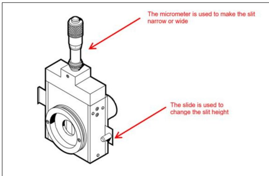
**Figure 10: A Micrometer Adjustable Slit.**
