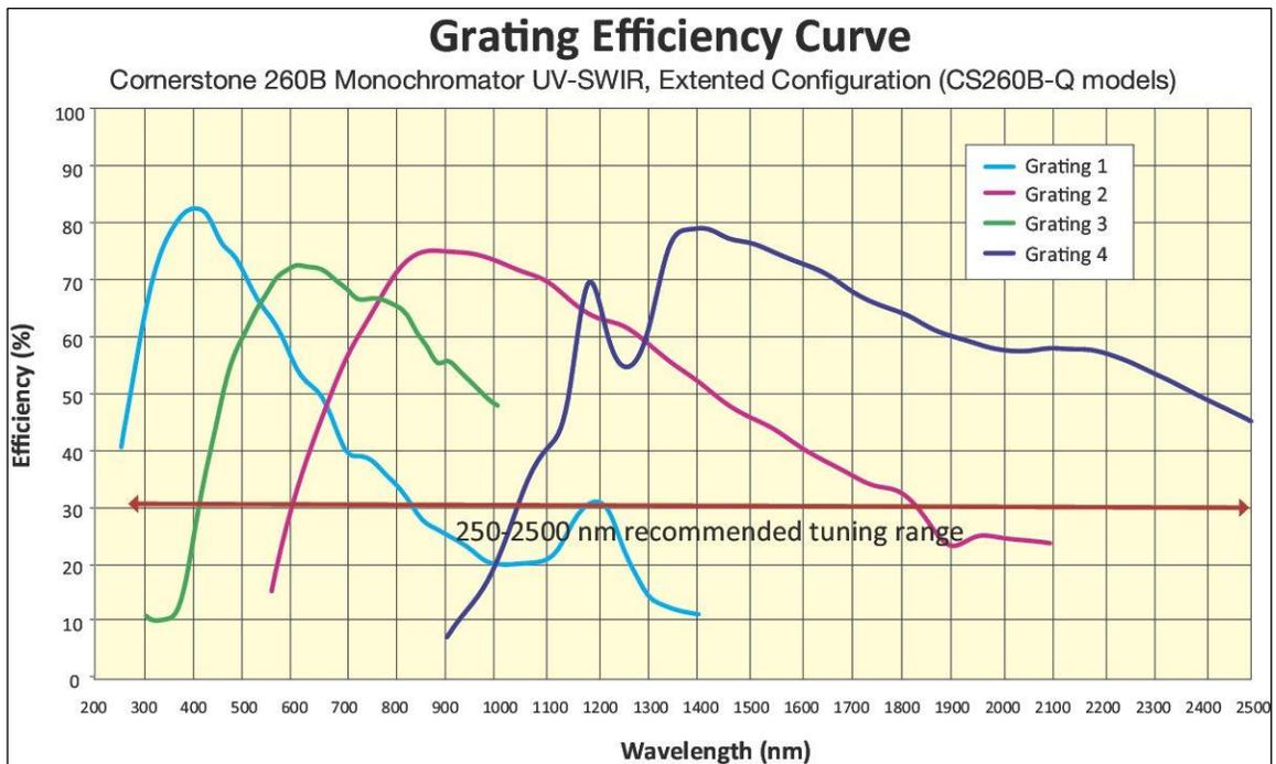
Figure 20: Grating Efficiency Curve, Cornerstone 260B Monochromator UV-SWIR, Extended Configuration (CS260B-Q Models).
