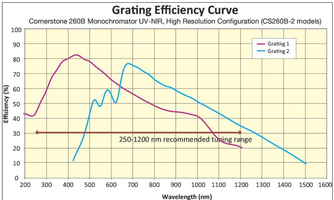
Figure 18: Grating Efficiency Curve, Cornerstone 260B Monochromator UV-NIR, High Resolution Dual Configuration (CS260B-2 Models).
