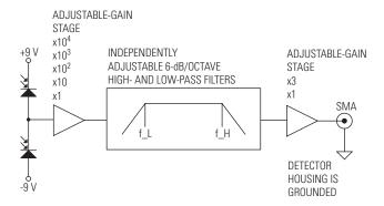
The following table summarizes the bandwidth at each gain setting. The bandwidth on the 3x settings is somewhat lower than the 1x settings, and significantly decreases at the highest gain settings. There is little difference in frequency response between the visible (Model 2107) and IR (Model 2117) models. The plots of Figure 3 show the frequency-response details for each gain setting.
