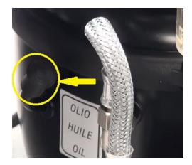
Figure 2 Remove rubber plug on the oil pipe
