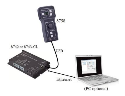
Figure 10 Single Controller Setup
