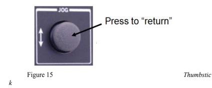
There are 20 distinct jog speed settings which can be customized by the user to best suit the application needs. The factory default settings start at 1 step/second and end at 2,000 steps/second – unless the Picomotor is of type 'Tiny', in which case the speed is automatically constrained by the controller to 1750 steps/second (max.).
