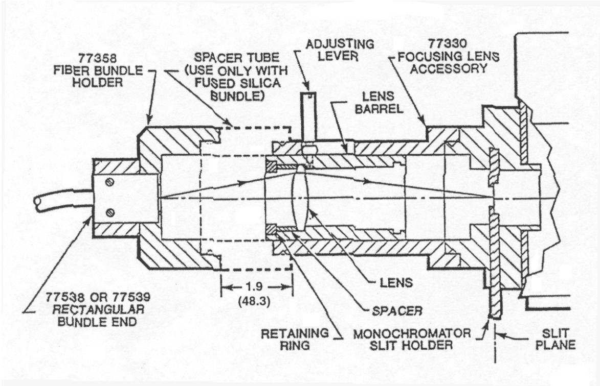
Figure 1 Coupling the Fiber Bundle to the Monochromator with the 77358 and 77330.
