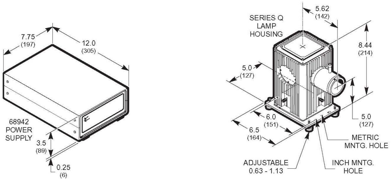
**Figure 3 : Dimensional diagram of 66080 Deuterium Source components**
