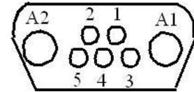
**Output Connector Pin Assignment**
