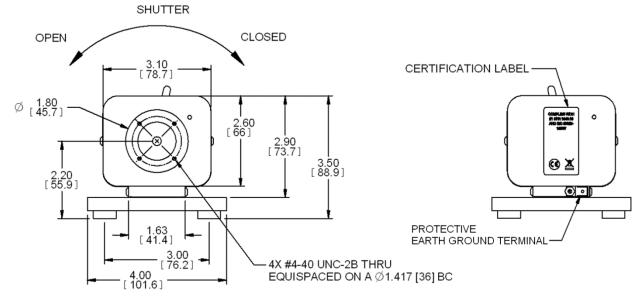
RECOMMENDED MOUNTING (WITH FEET) 4X Ø.25 GROMMET THRU HOLE
