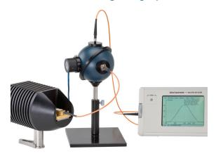
Complete your integrating sphere set-up with a wide variety of accessories that make interfacing fibers and detectors easy.
