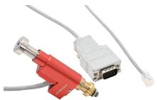
If instead you're going to mount the motor's shaft in a micrometer clamp, be careful not clamp too hard on the motor's housing. This can deform the motor's shank and may cause in-creased friction between the inner rotating screw and the fixed exterior housing. If the motor slows or fails completely, try loosening the clamp.
