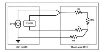
FIGURE 2 – Recommended Three-Wire Configuration
