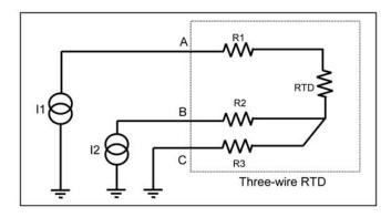
FIGURE 1 – Three-Wire RTD System
