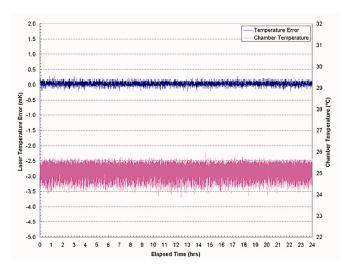
FIGURE 3 – Temperature Error
