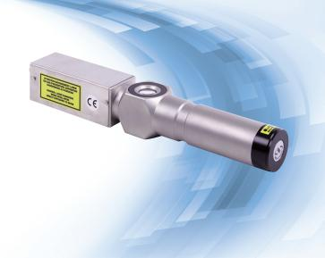
The CONEX-LDS autocollimator performs high-resolution, non-contact angular measurements for alignment, quality assurance and metrology applications. The controller is integrated in the body of the autocollimator making it ideal for systems integration or as a portable metrology tool. The CONEX-LDS is used in the highest precision applications performing high resolution angular measurements at over distances of up to 5 meters.
