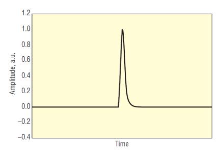
Figure 7. Time-Domain Optimized: This is the impulse response of a detector that is optimized for the time domain. You can see the characteristic frequency response in the figure above.
