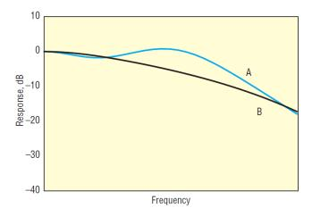
Figure 6. Frequency-Domain vs. Time-Domain: (A) Detectors designed for flat frequency response have enhanced responsivities at high frequencies. (B) Detectors that are optimized for clean, ring-free pulses show a characteristic drop off in 3-dB frequency response.
