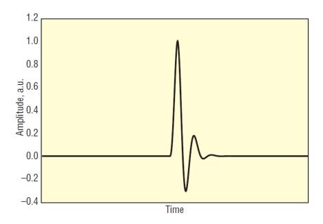
Figure 8. Frequency-Domain Optimized: This is the impulse response of a detector that is optimized for a flat frequency response. You can see the corresponding frequency response in figure above.
