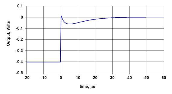
Figure 9. Example crossover behavior for DC-coupled receivers.
