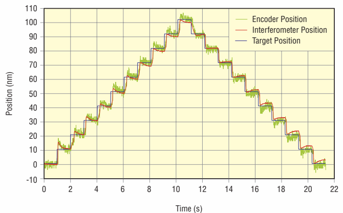
VP-25XL stages deliver 10 nm motion sensitivity with high reliability and position stability.
