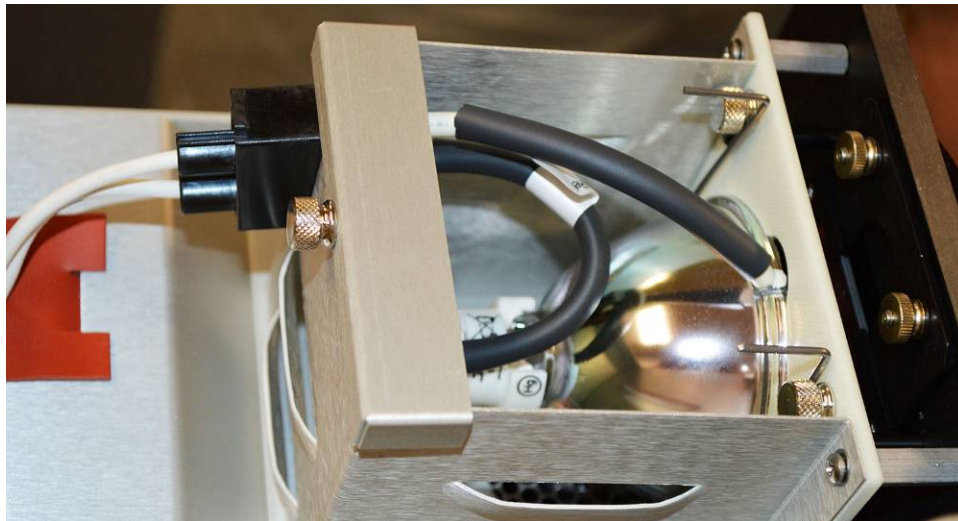
Figure 16: Lamp mounted properly in its cage
