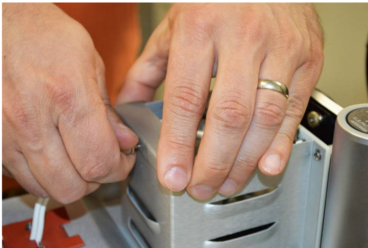
Figure 10: Lamp cage retention cover and thumbscrew
