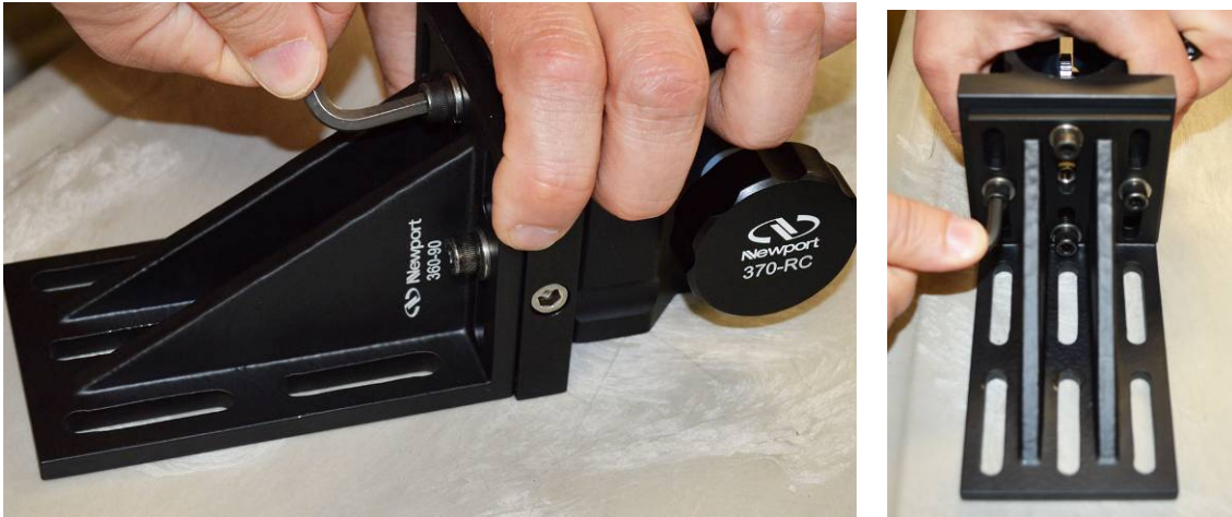
Figure 4: 90 Degree angle bracket to Post Clamp assembly
