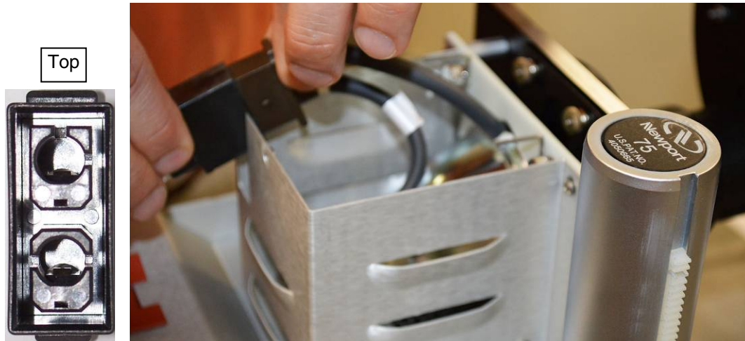
Figure 15: Lamp connector engagement
