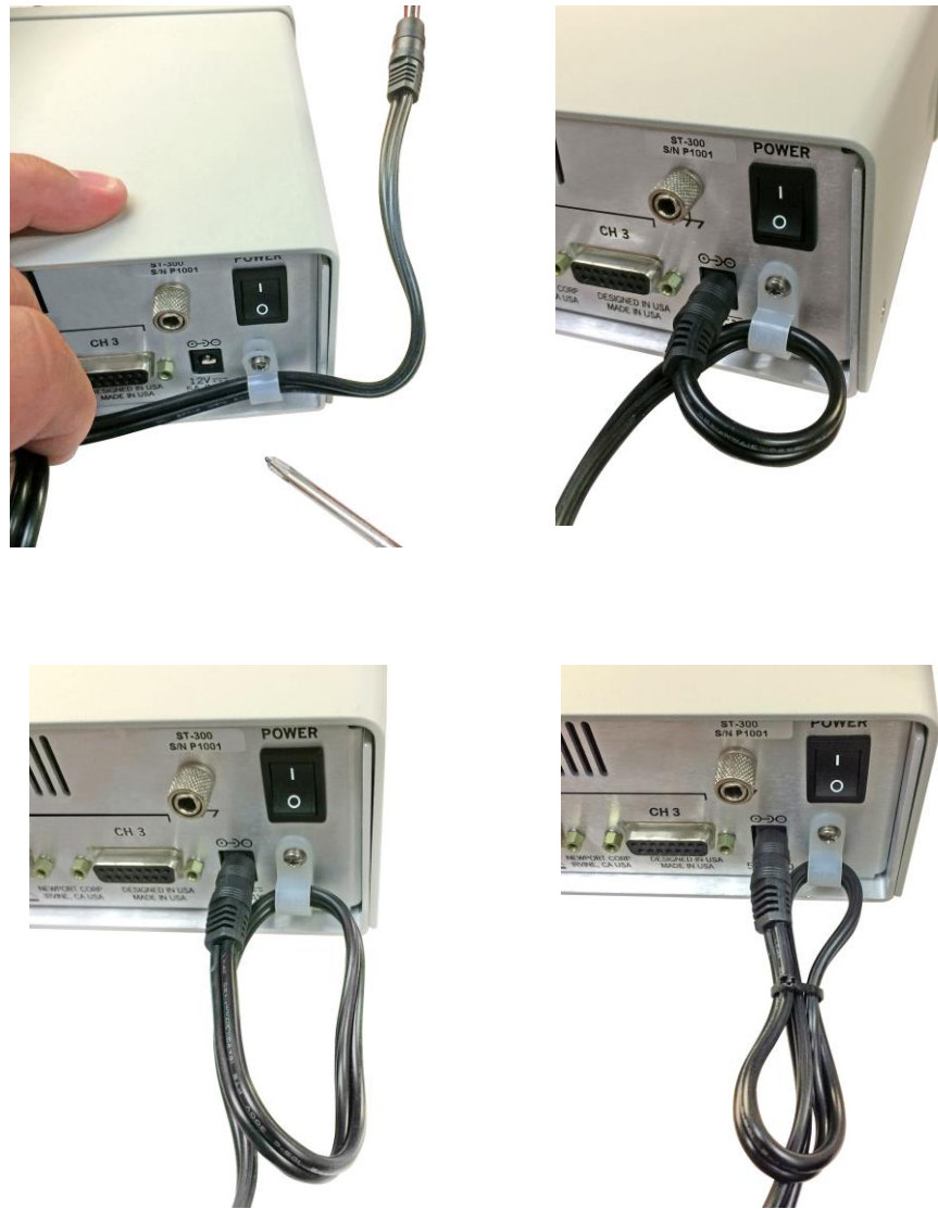
Figure 13 Optional strain relief to secure the power cord
