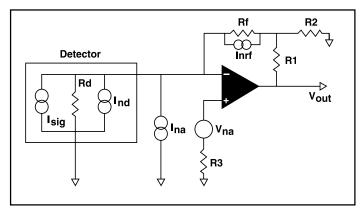
Figure 1. OMH-6709B Receiver Circuit.
