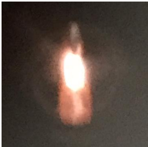
Figure 47: Xe arc lamp output with primary arc image centered.
