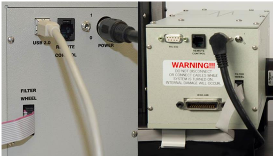
Figure 16: For the TLS-300XU and TLS250QU, connect a USB 2.0 cable into the USB port on the side of the monochromator. For the TLS-300XR and TLS250QR, connect a RS-232 or GPIB cable into the properly labeled port on the side of the monochromator.
