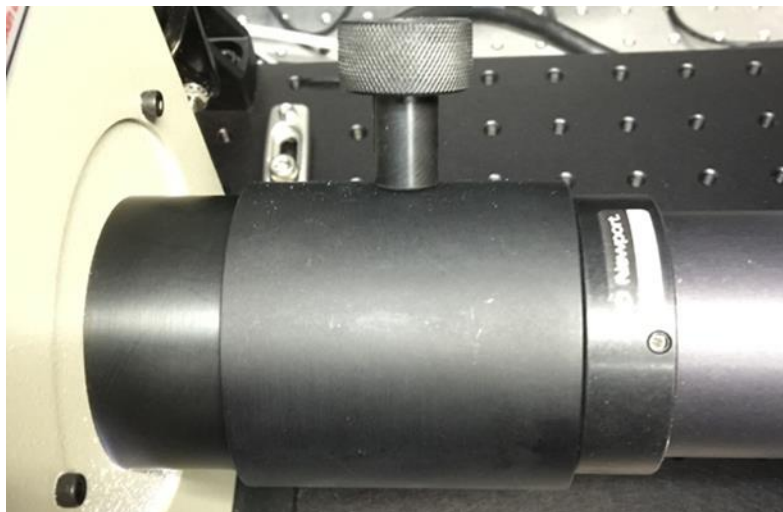
Figure 39: Condenser lens assembly adjustment knob and adjustment lever at output of lamp housing.
