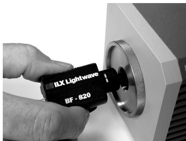
Figure 2.12 – Inserting the BF820
