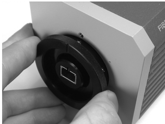
Figure 2.6 – Seating the Alignment Pin
