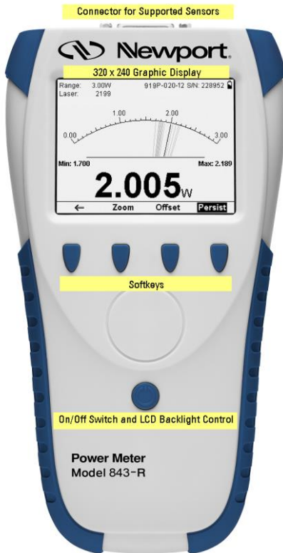
Figure 3.1 843-R displaying power measured with a Thermopile sensor. Displayed in analog needle mode with persistence on.
