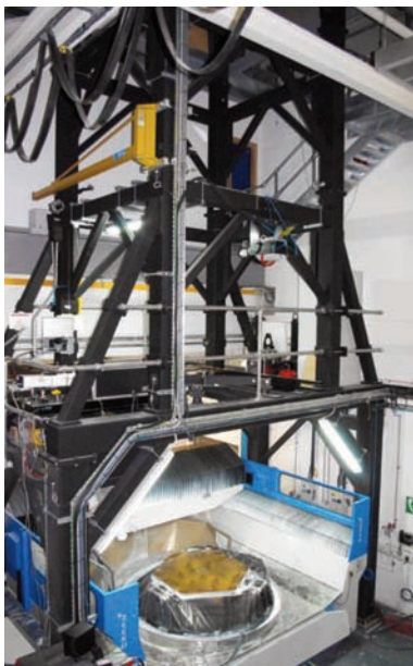
Figure 2: Optical Mirror Polishing Tower for the E-ELT (Courtesy of OpTIC Glyndwr Ltd and Glyndwr University)
