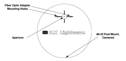
Figure 2.4 OMH-6703B Optical Measurement Head
