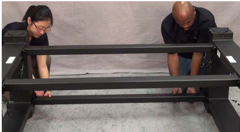
Figure 4 Connecting cross-braces to INT leg weldments
