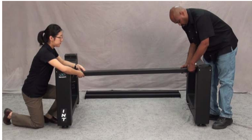
Figure 2 INT leg weldments and cross-brace positioning
