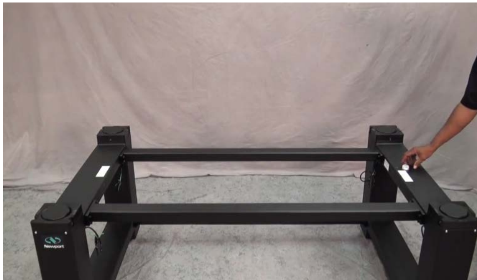
Figure 6 Completed INT frame assembly
