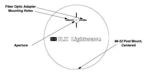
Figure 2.4 OMH-6727B Optical Measurement Head
