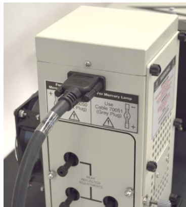
Figure 6 The electrical connector on an Oriel Research Lamp Housing for use with an OPS-Q Model Power Supply.
