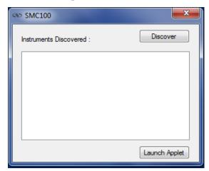
Next, click on "**Discover**" button and the number of instruments discovered will appear. This window allows the user to select a com port where the desired instrument is connected.
