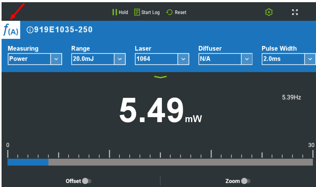
Figure 9-2 Pyroelectric Power Bargraph
