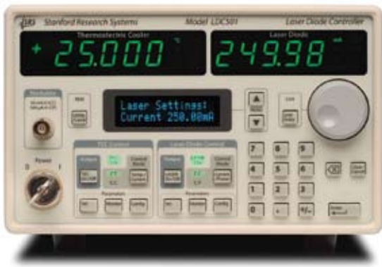
FIGURE 2. In addition to current control, controllers add temperature control, typically a thermoelectric cooler (TEC), to cool the heat output from the diode. The LDC501 laser-diode controller from SRS offers dynamic switching between constant current and constant power modes, with a dedicated front-panel display for parameter entry (left). The Thorlabs LDC 200 series of controllers provides currents ranging from 20 mA to 4 A in seven models with temperature stability of better than 500 ppm/°C (below).
