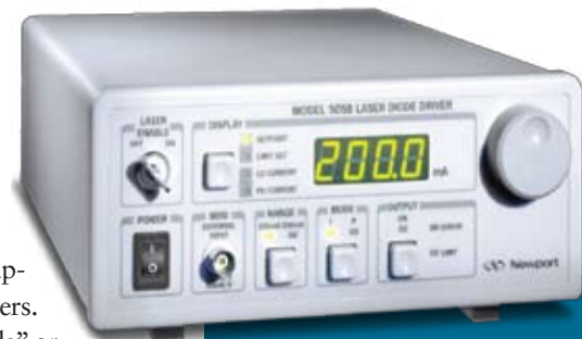
FIGURE 1. Drivers provide the operating current entering a system. The 500B series laser-diode driver from Newport (above) is a low-noise current source with long-term stability of better than 50 ppm/°C with four models covering laser currents from below 50 mA up to 6 A. A USB 2.0 connector interface is unique for interfacing with a remote computer. The LDX36000 family of high-power laser-diode current sources from ILX Lightwave (below) provides continuous-wave and pulsed operation with currents up to 220 A and voltages to 70 V for driving stacks and arrays of lasers.
