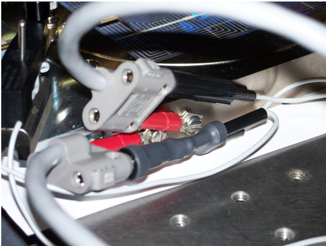
Figure 7: Using 90026574 and 90026575 adaptors to connect to the vacuum chuck
