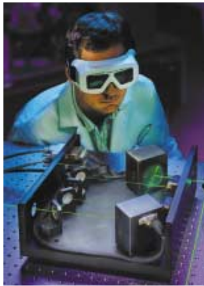
FIGURE 3. Beam-stabilization module incorporates two high-performance FSMs (0.55-kHz bandwidth) working with two quadrant detectors to provide closed-loop tilt compensation.
