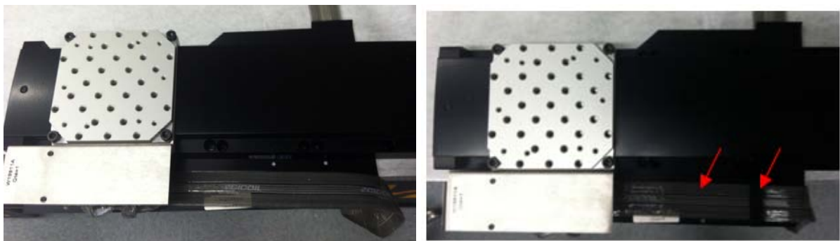
Figure 6. Y-Stage Cable on Y-Support Bracket
