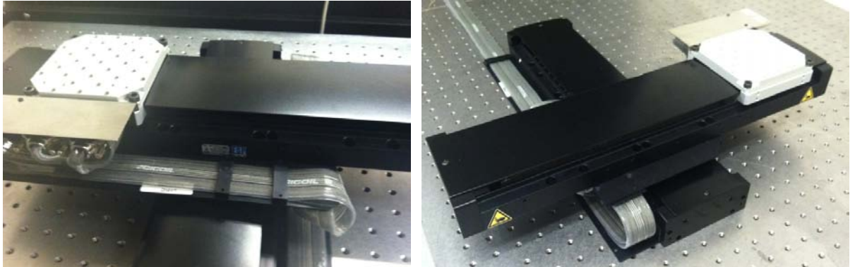
Figure 7. Y on top of the X-Stage, Cable Routing.
