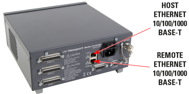
Figure 15: Direct connection to the ESP302 using Ethernet cable.
