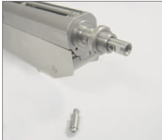
Ball tip of the LTAHSPPV6 actuator.
